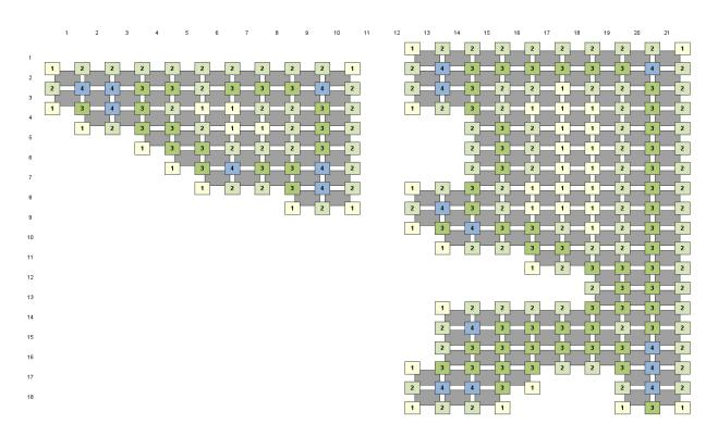
Note: Blocks above with values greater than 4 require extra ballast bays. The proper number of bays are provided in the Bill of Materials. The installer must install these extra bays as near to the indicated location as possible.
