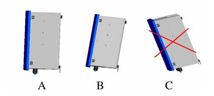
Figure 4-1 Digiwatts unit mounting positions
