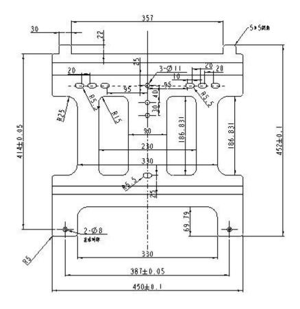
Figure 4-3 Dimensions of the Wall Mounting Bracket
