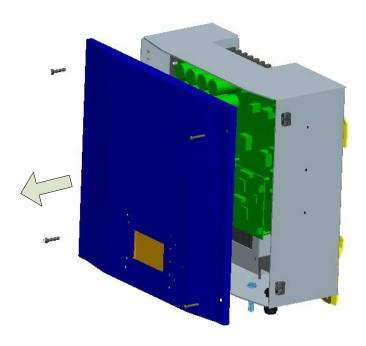
Figure 3-1 Opening the Digiwatts Unit
