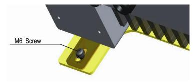
Figure 4-6 Affix Bottom Tabs of Digiwatts unit to Mounting Bracket.
