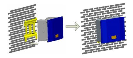
Figure 4-5 Attach the Inverter to Bracket
