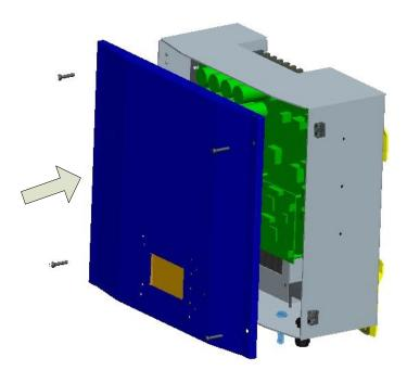
Figure 5-8 Closing the Digiwatts unit
