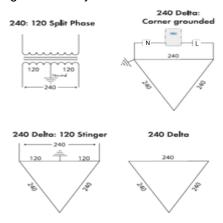
Figure 3-3: Common Utility Voltage Configurations
