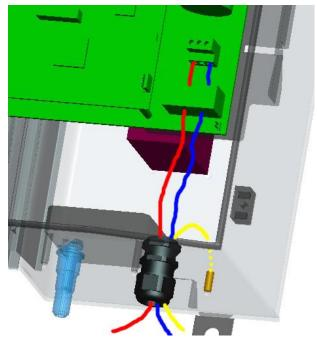
Figure 5-3 AC Connection Terminals
