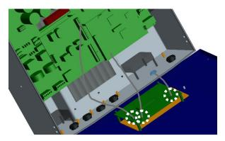
Figure 5-2 (b) Front Cover Electrical Connections
