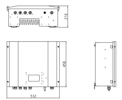
Figure 1-4 Dimensions of the Digiwatts unit
