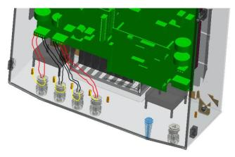
Figure 5-5 DC Connection Terminals
