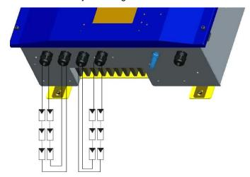
Figure 5-4 PV Modules Connection to Digiwatts unit
