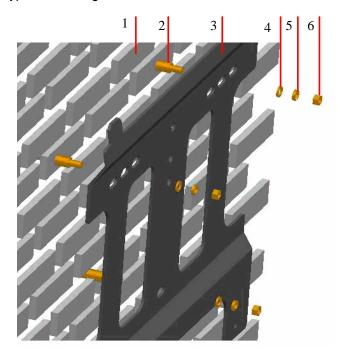
Figure 4-4 Fasten the Bracket against Masonry Wall with Expansion Screws
