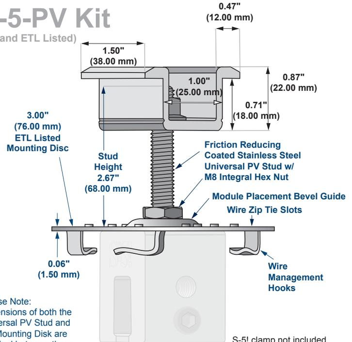
Please Note: Dimensions of both the Universal PV Stud and the Mounting Disk are identical between these two illustrations.
