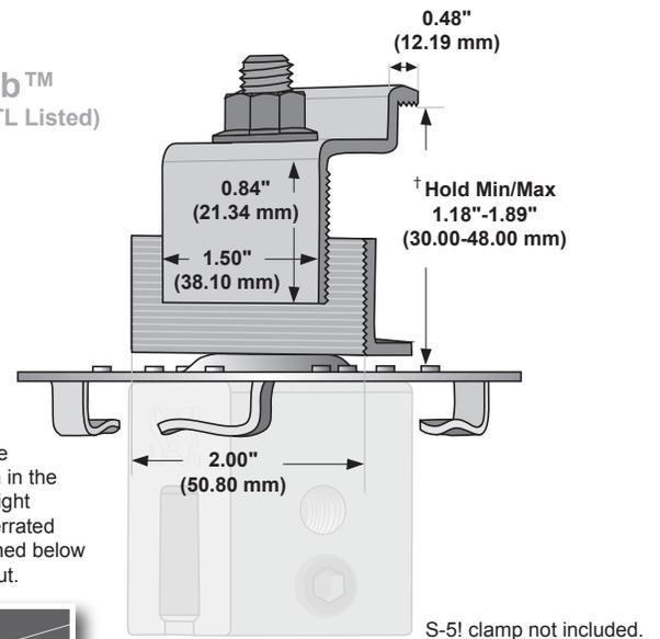
Please note: The assembly option in the diagram to the right illustrates the serrated L-flange positioned below the stud's hex nut.
