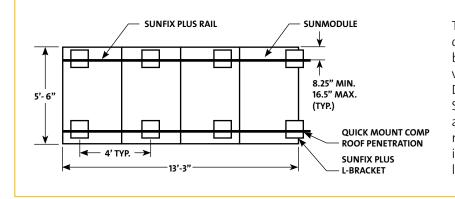
The pre-engineered Sunkits are designed with 4 portrait module building blocks for maximum versatility with common components<sup>3</sup>. Due to the high versatility of the Sunfix plus mounting solution, alternate layouts are possible. The most common layout options are included in the standard racking layout provided.
